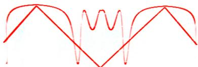
WF 3 has an extra clipping stage that follows and squares up OUT 3. This is the PULSE output and it can be used to trigger and/or gate modules requiring such, as well as be used as an audio source. The output range is approx. 0-7V.
